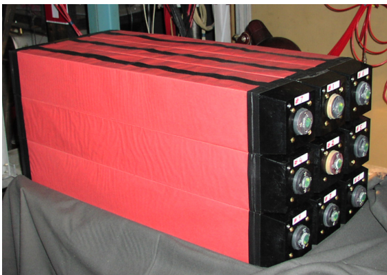
Figure 2.12: 3 \times 3 matrix of prototype Shashlyk modules as they should be employed for the PANDA Forward Electromagnetic Calorimeter.
