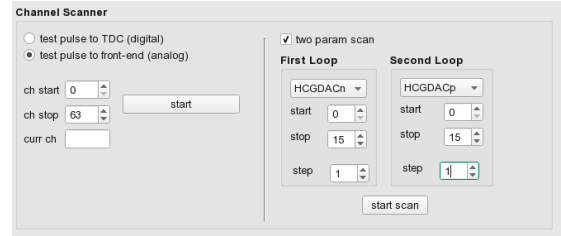
Fig. 7. GUI widget to automatize the procedure to test the chip.
