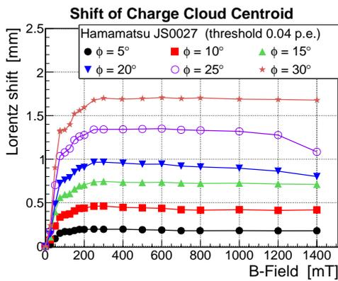
Figure 3: Lorentz shift for different tilt angles  $\phi$  measured inside the new 2-inch  $6 \times 128$  pixel Hamamatsu R13266-M768 MCP-PMT.
