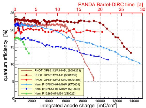
Figure 4: Comparison of the results of our lifetime measurements for different ALD coated MCP-PMTs: QE as a function of the IAC at 400 nm.
