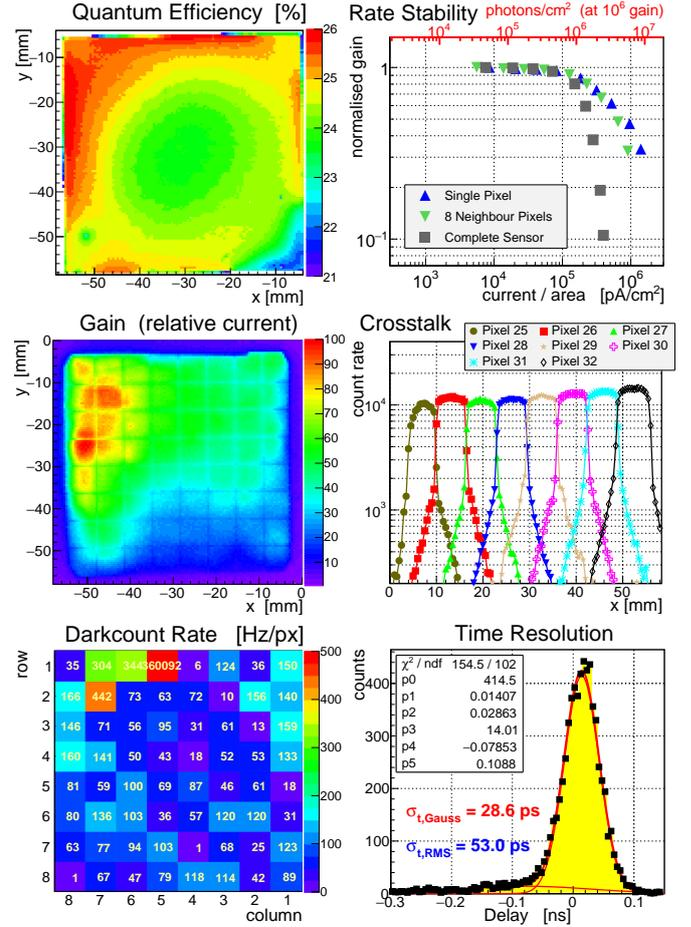
Figure 1: Compilation of the most important properties of the new 2-inch  $8 \times 8$  pixel Hamamatsu R13266-M64 MCP-PMT JS0035.
