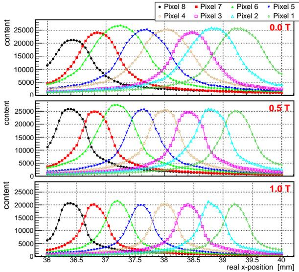
Figure 2: Response of eight adjacent pixels of the new 2-inch  $6 \times 128$  pixel Hamamatsu R13266-M768 MCP-PMT as a function of the photon position outside and inside a magnetic field.
