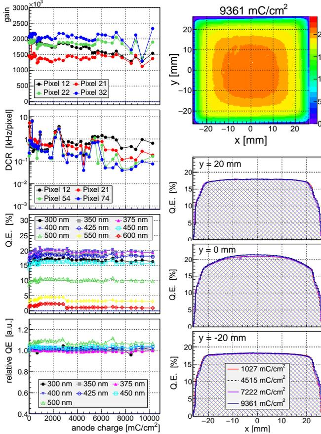
Figure 5: PHOTONIS MCP-PMT XP85112 (9001393); left column: gain, dark count rate (DCR), absolute QE for different wavelength, and relative QE normalized to 350 nm as a function of the IAC; right column: xy-scan of the QE of the PC surface at 9.36 C/cm<sup>2</sup> and QE projections at three y-positions at 4 different IACs. 240
