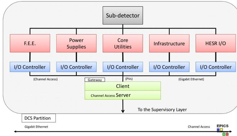
**Figure 2.** DCS Partition for one sub-detector. The partitions are build up of the field layer (red), control layer (blue), and the CA gateway (green).
