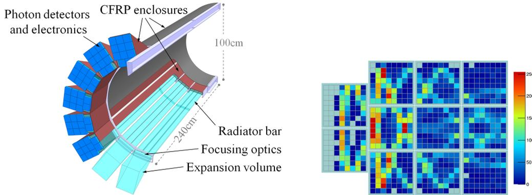
**Figure 2.** Left: Schematic of the Barrel DIRC baseline design. Only one half of the detector is shown. Right: Geant simulation of the baseline geometry of the PANDA Barrel DIRC. The colored histogram shows the accumulated hit pattern from 1000  $K^+$  at 3.5 GeV/c momentum and  $55^\circ$  polar angle.
