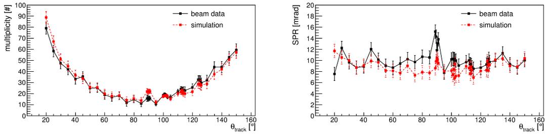
**Figure 3.** Photon yield (left) and SPR (right) as a function of the track polar angle for the narrow bar and the 3-layer spherical lens for tagged protons at 7 GeV/c beam momentum in data (black) and Geant simulation (red). The error bars correspond to the RMS of the distribution in each bin. The use of lower-quality, older sensors affected predominantly the angles around 90° (left and right).
