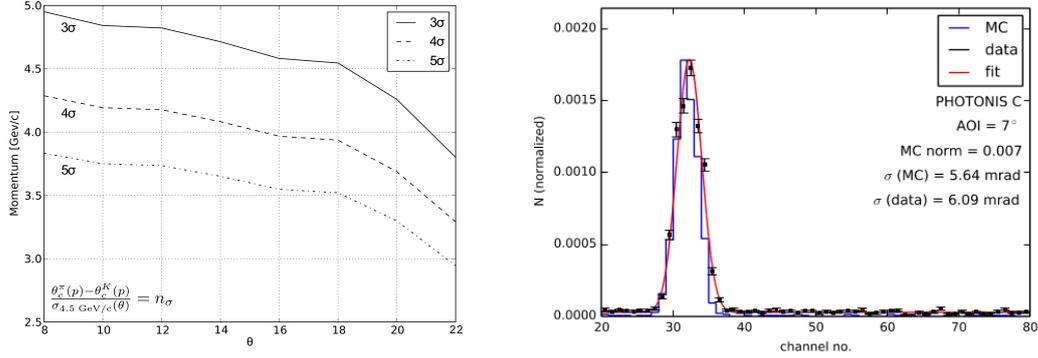
**Figure 5.** Left: Pion/kaon separation computed from the distribution of reconstructed Cherenkov angles for a ROM consisting of a 2'' tube with 0.5 mm pixel width. Right: Comparison of data and Monte-Carlo of the single-photon resolutions at 10 GeV/c beam momentum.
