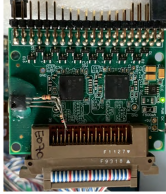
Figure A.1: A prototype FEB for FT read-out with bonded PASTTREC ASIC and DS18s20 temperature sensor mounted.
