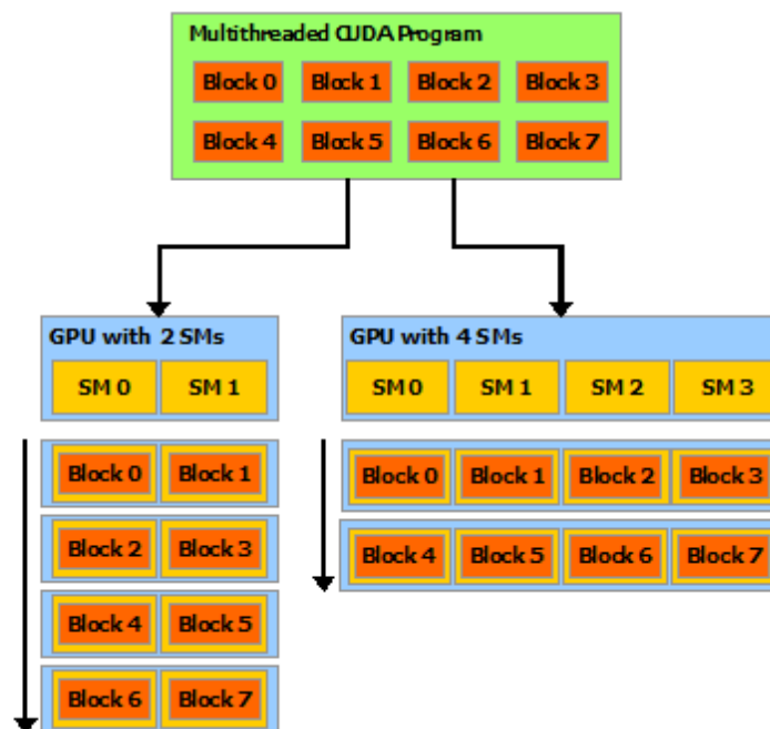
FIGURE 5.9: CUDA program block structure. Each block is assigned to one SM for processing [127]. Depending on the number of SMs in the GPU more blocks can be processed in parallel.
