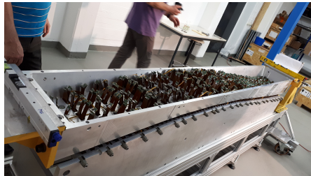
Figure 16. Assembly of the first slice of the \bar{P} ANDA barrel calorimeter including the support-beam (right picture).
