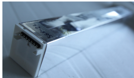
Figure 13. Finished single crystal-unit with reflector and capsule on top of the APDs. After this step each unit will be inserted into the carbon fiber alveoli.
