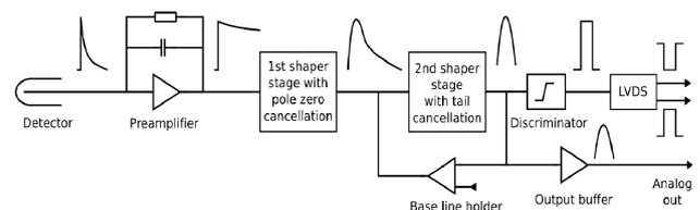
Figure 1: Block diagram of the PASTTREC chip.
