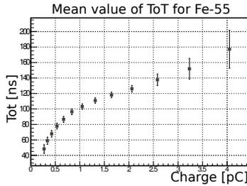
Figure 2: Time-over-threshold and charge correlation. Data taken with a  $^{55}\text{Fe}$  source. The correlation is used to translate the ToT to charge values.
