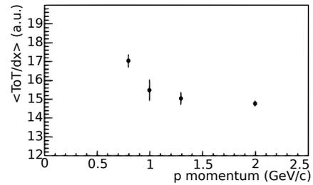
Figure 4:  $\text{ToT}/dx$  for different beam momenta.
