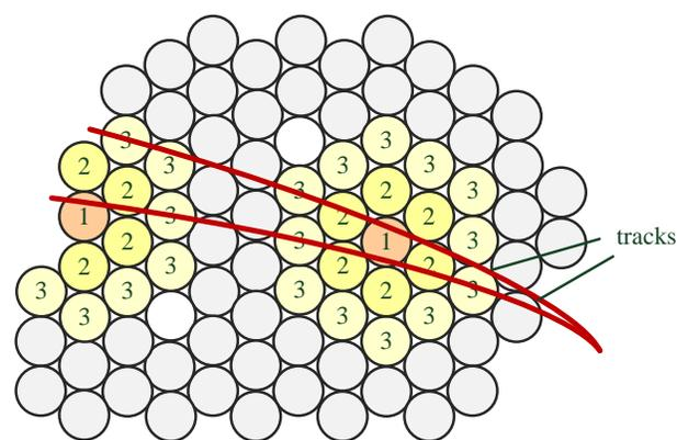
Fig. 12. Event filtering. If an event takes place in cell 1, the event presence in the neighboring cells denoted by 2 and 3 will be checked.
