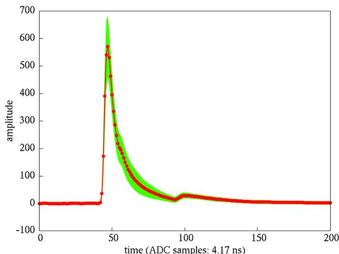
Fig. 4. Sampled response to  $^{55}\text{Fe}$  irradiation using an increased shaping time due to cabling. The solid line shows the mean value, while the shaded band indicates the standard deviation. A small second peak is related to signal reflection at the amplifier, which is located at the end of 20 m cable.
