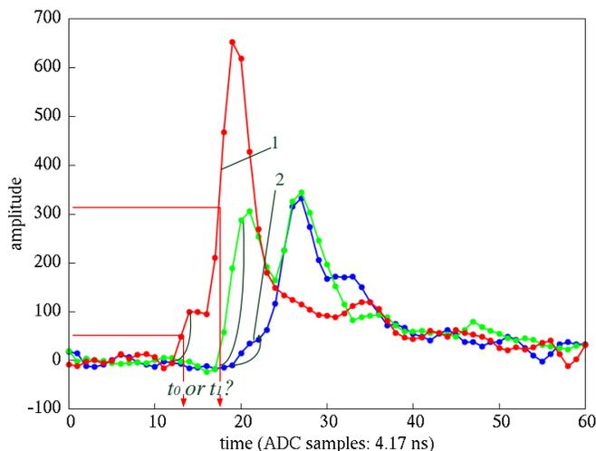
Fig. 9. Sampled responses of 4 straws showing that only a few points on the leading edge are taken into consideration.
