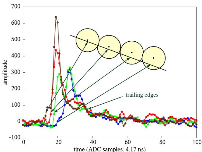
Fig. 8. Responses of four straw tubes to the same particle track.
