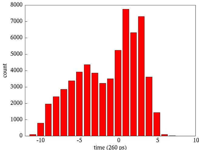
Fig. 3. Distribution of differences (in bins of 260 ps) between the constant fraction times measured with the sampling rates of 120 MHz and 240 MHz for  $^{55}\text{Fe}$  irradiation. The root mean square (RMS) value of the distribution is 1.04 ns.
