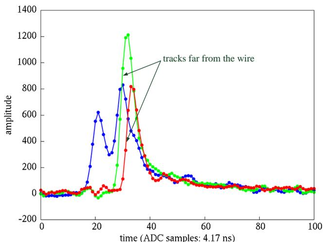
Fig. 11. Sampled responses of the track near the wire and far from the wire.
