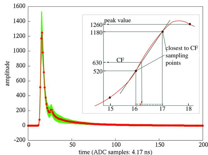
Fig. 2. Sampled response to  $^{55}\text{Fe}$  irradiation. The solid line shows the mean value averaged over 60,000 responses, while the shaded band indicates the standard deviation. The inset illustrates the constant fraction method with linear interpolation of the rising edge through the two sampling points closest to the threshold value denoted by CF.
