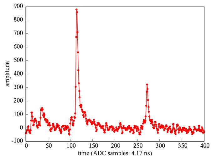
Fig. 7. Response to multiple particle tracks crossing a straw tube by proton beam irradiation.
