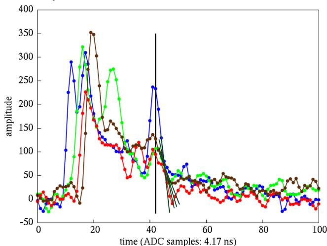
Fig. 10. Sampled responses of a track near the wire. The vertical line indicates the mean position of the last maximum, while the short straight lines show the linear interpolation of the trailing edges. The trailing edge slopes cross in a small region. The last maximum position is not the same.
