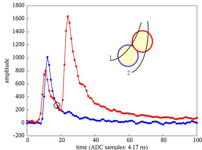
Fig. 15. Double track resolution. Signal pile-up leading to incorrect time measurements.
