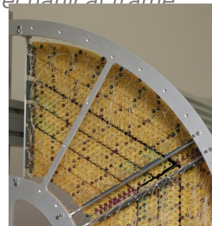
Hexagon sector, mounting brackets to fix modules in mechanical frame
