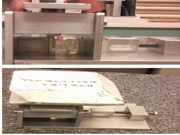
Figure 5.3: Set-up for testing the mechanical resistance. The white metal block (on the bottom) induces the mechanical force.
